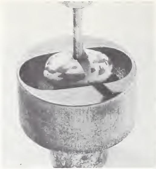
Figure 2. A single unit of the bean cooker, showing plunger and bean in place.
